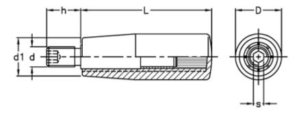
$$\begin{array}{ll} D & = 21 \\ d1 & = 17 \\ d \ 6g = M6 \\ h & = 13 \\ L & = 50 \\ s & = 3 \end{array}$$
